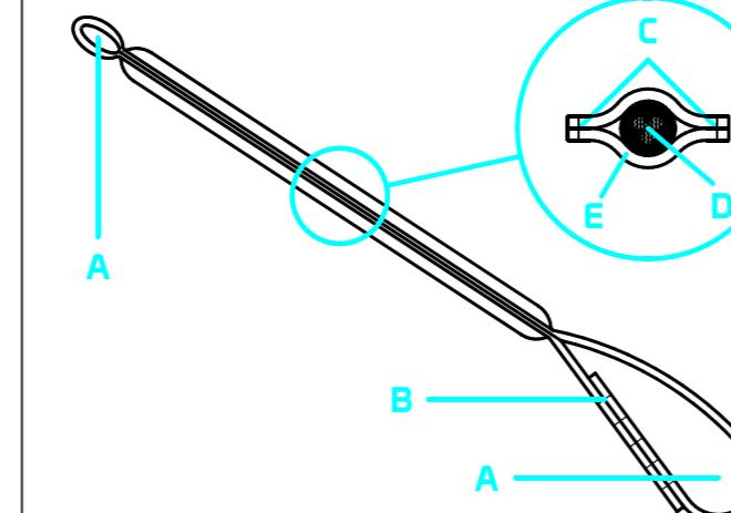
**EN:** (A) Loop, (B) Main stitching, (C) Secondary stitching, (D) Stiffening cable, (E) Tape.
