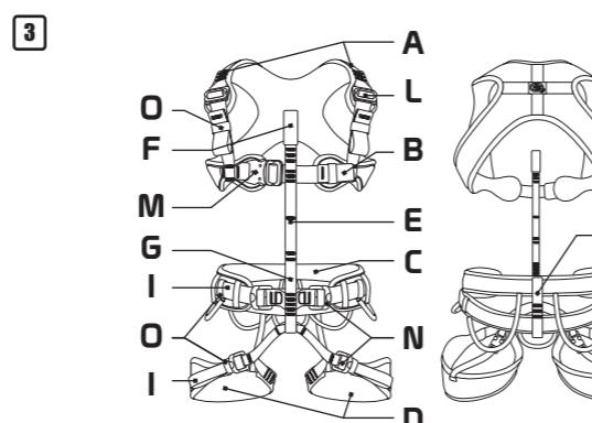
EN: (A) Shoulder straps, (B) Sternal sling, (C) Waist belt, (D) Sit harnesses, (E) Connection sling, (F) Sternal attachment point, (G) Ventral sling attachment point, (H) Back attachment ring, (I) Adjustment slings, (L) Buckles in aluminium alloy, (M) Quick-release automatic buckle in aluminium alloy, (O) Buckles in carbon steel, (O) nylon or polyester Loops. Unless otherwise specified, the textile parts are made of polyester.
