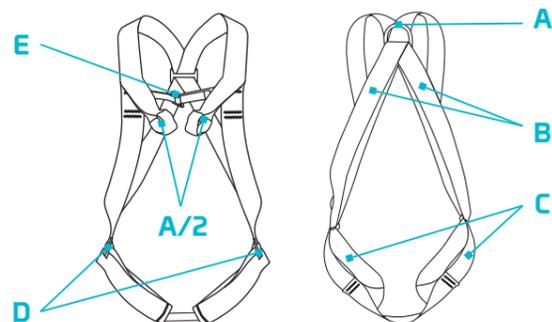
**EN:** (A) Dorsal attachment point, (A/2) Sternal attachment elements, (B) Shoulder straps, (C) Thigh loops, (D) Adjustment buckles, (E) Sternal sling and buckle.
