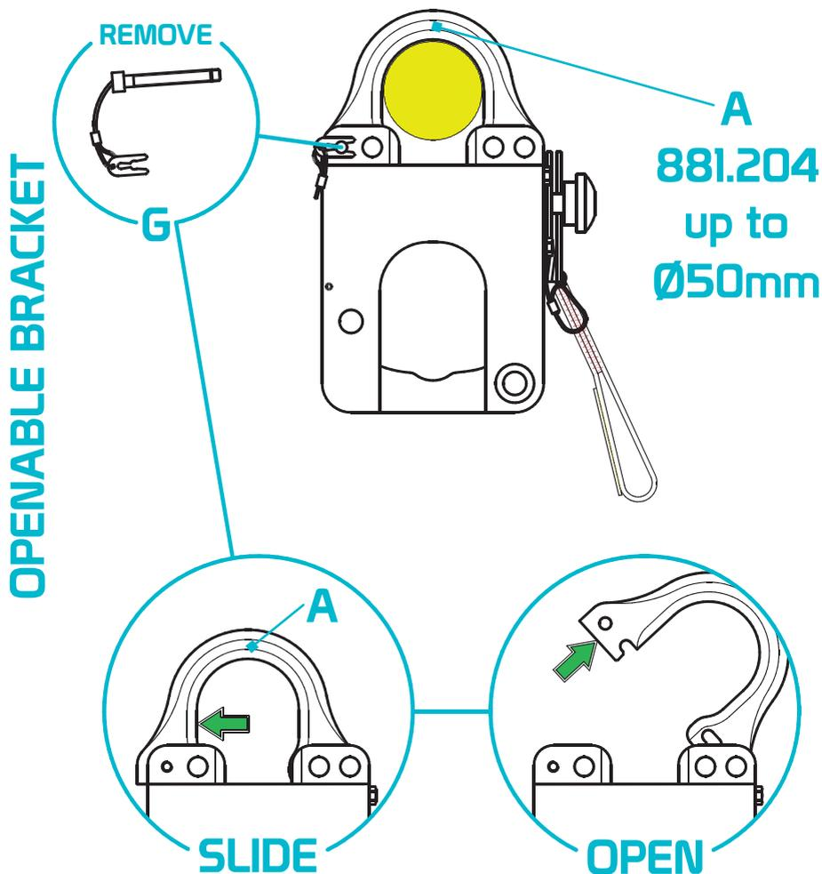
**Fig. 5 – Release** – It is required a slight force applied to the lever (B) to open the device:
