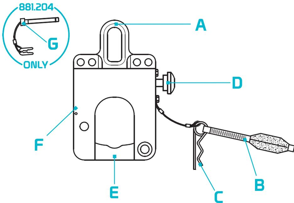
(A) Bracket, (B) Strap, (C) Safety pin, (D) Release button, (E) Gate, (F) Lever, (G) Closing screw.
