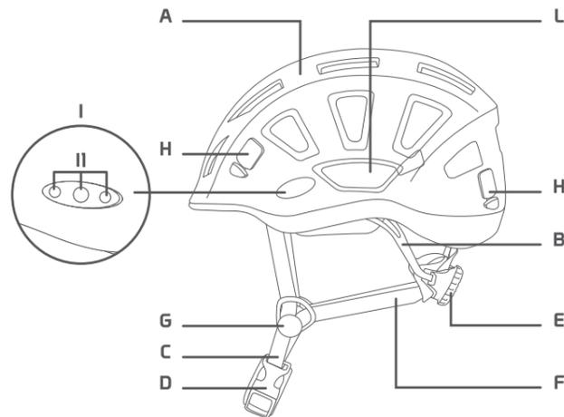
A Shell | B Head band | C Chin strap | D Buckle | E Size adjustment system | F Side slings | G Dividing buckles | H Lamp holders | I Protective insert | II Visor and torch "SIDE LIGHT" fixing holes | L Earmuffs fixing hole
