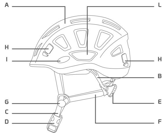
**A** Shell | **B** Suspension harness | **C** Chin strap | **D** Buckle | **E** Size adjustment system | **F** Side slings | **G** Dividing buckles | **H** Lamp holders | **I** Visor fixing hole | **L** Earmuffs fixing hole
