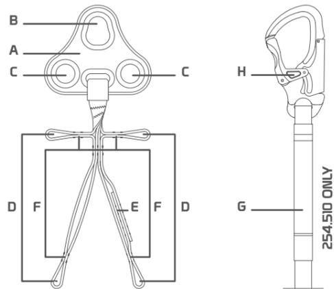
**A** Plate | **B** Main hole | **C** Secondary holes | **D** Eyelets | **E** Main seam | **F** Secondary seams | **G** Tear-off seams (only 254.S10 version) | **H** "double gate" connector 715.0X0 TANGO (only 254.S10 version)
