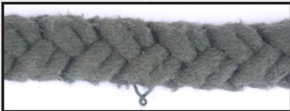
**Picture 2: Hooked yarn under 25mm**
