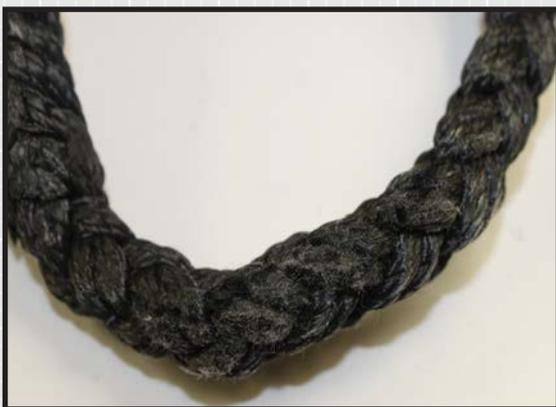
Picture 11: Normal surface abrasion on extraction loop.
